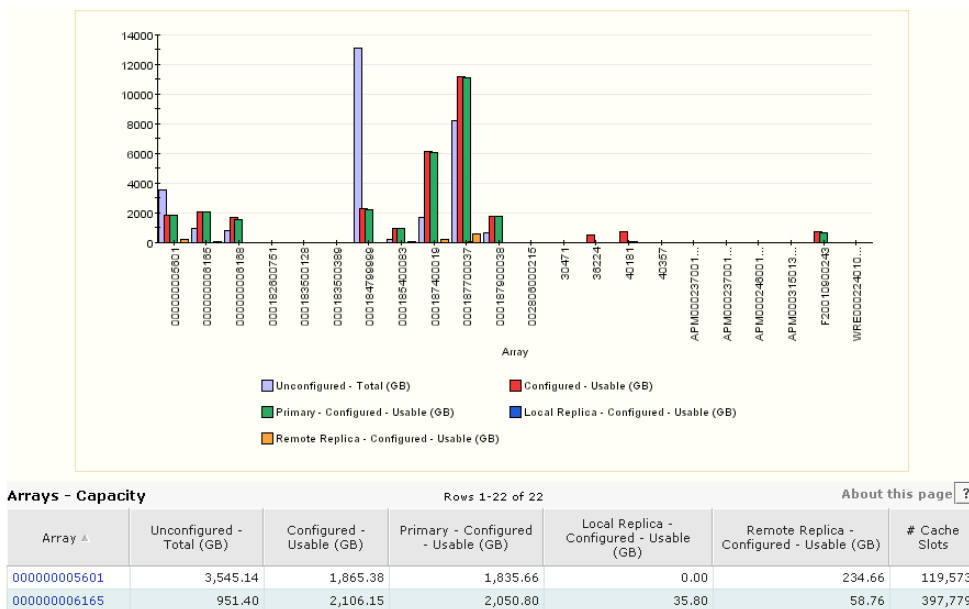
Figure 5-4 Effective Array Capacity Graph
