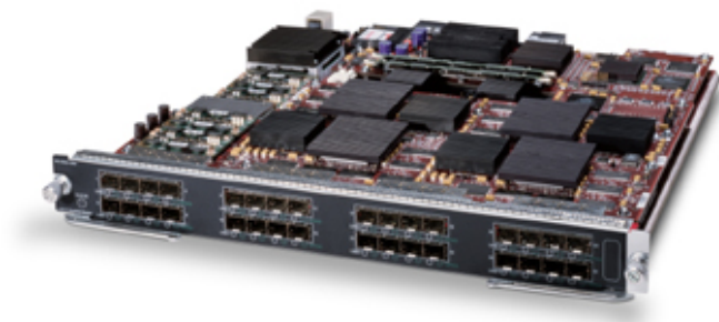
Figure 7. Cisco MDS 9000 Family Storage Services Module
