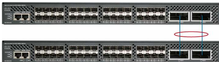
Figure 2. Cisco MDS 9134: Two Cisco MDS 9134 Switches Stacked Using 10GBASE Copper CX4
