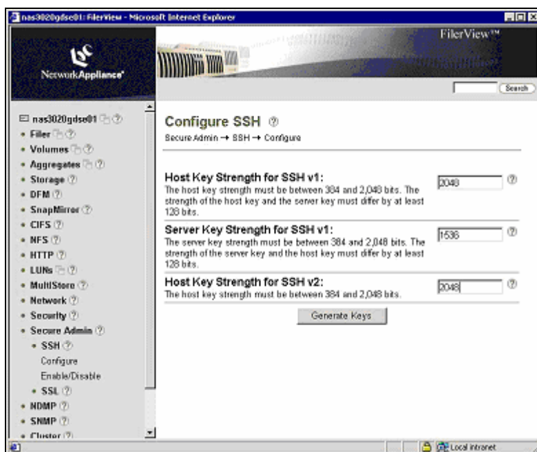
Figure 10.13 - NetApp FilerView - SecureAdmin SSH Configuration Screen
