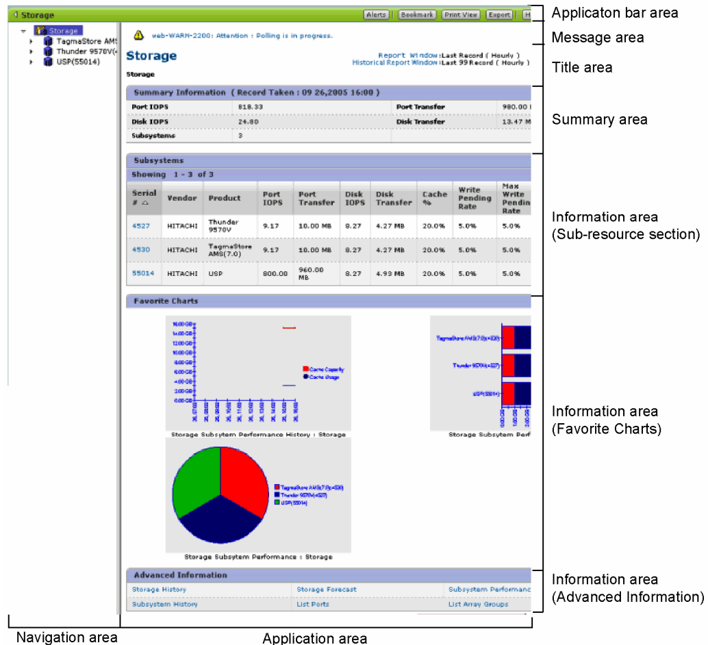
Figure 1.2 The Structure of the Report Area
