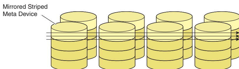
Figure 5. Protected Striped Meta Device on Eight Physical Disk Spindles
