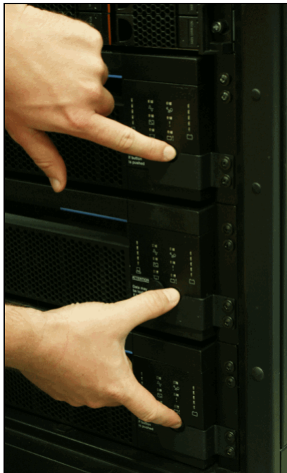
Figure 3-23 Use both hands to hit the three Test buttons simultaneously
