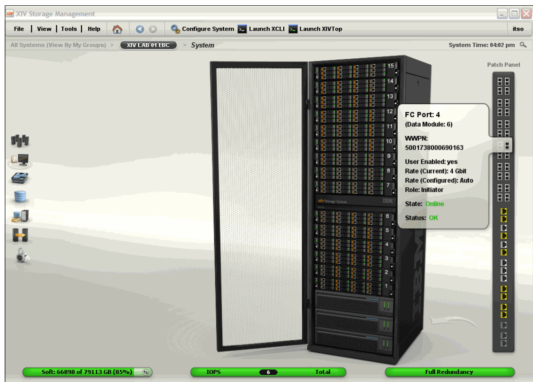
Figure 3-47 Port information from the patch panel view
