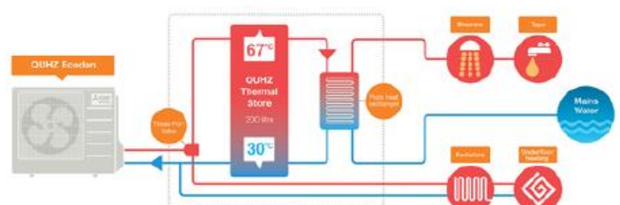
Thermal Store schematic
